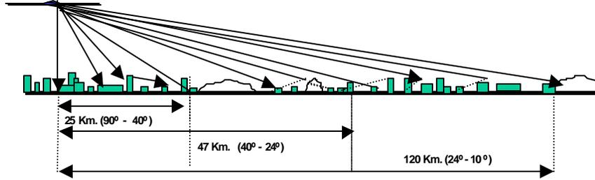
Fig.1. The HAPs communications scenario for the aeronautical channel.
