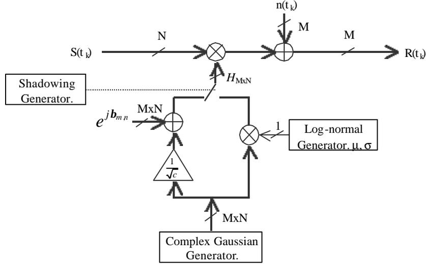
Fig. 2 MIMO channel model for simulation.
